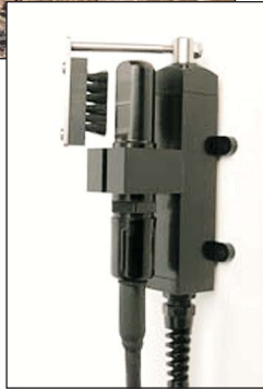
Hydro-Wiper protecting a Seapoint Turbidity Sensor from heavy biofouling
